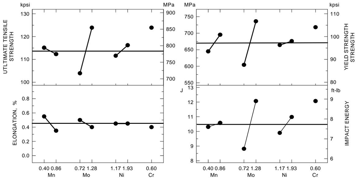
Figure 3. Mean effect of manganese, molybdenum, nickel and chromium on ultimate tensile and yield strengths, elongation and impact energy.
