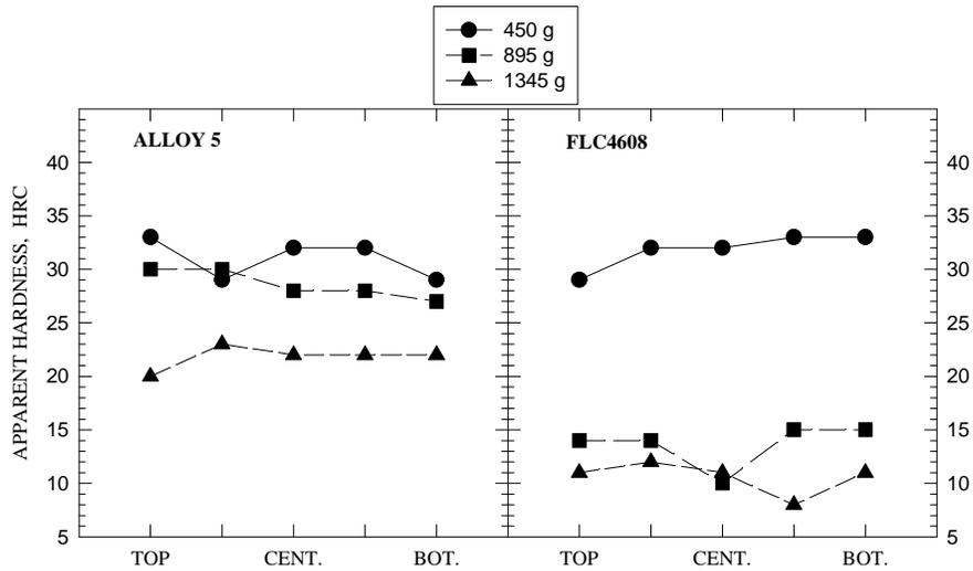
Figure 5. Apparent hardness measured on the cross section of disc specimens made from alloy #5 and a commercial FLC4608 material.
