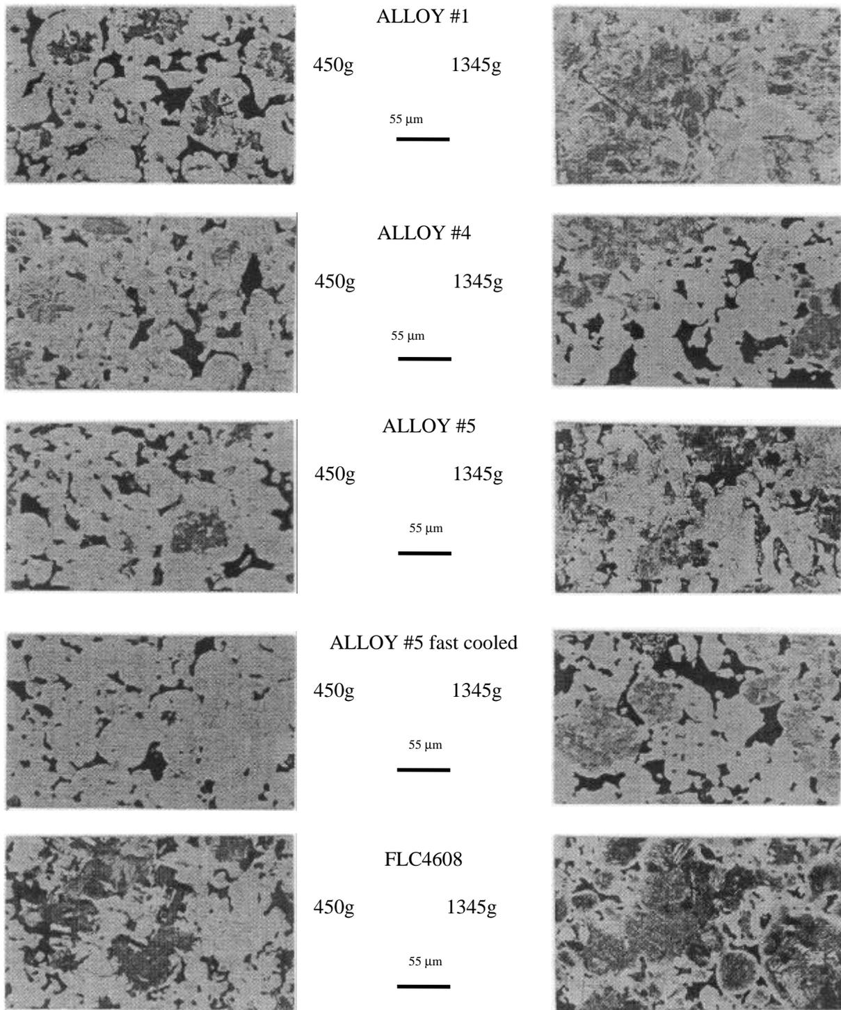
Figure 6. Microstructure of small (450g) and large (1345g) disc specimens made from alloys #1, #4, #5, fast cooled #5 and from a commercial FLC4608 mix.
