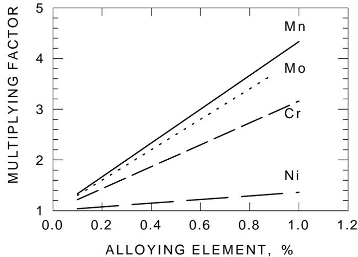
Figure 1. Hardenability multiplying factor of manganese, molybdenum, chromium and nickel [4].
