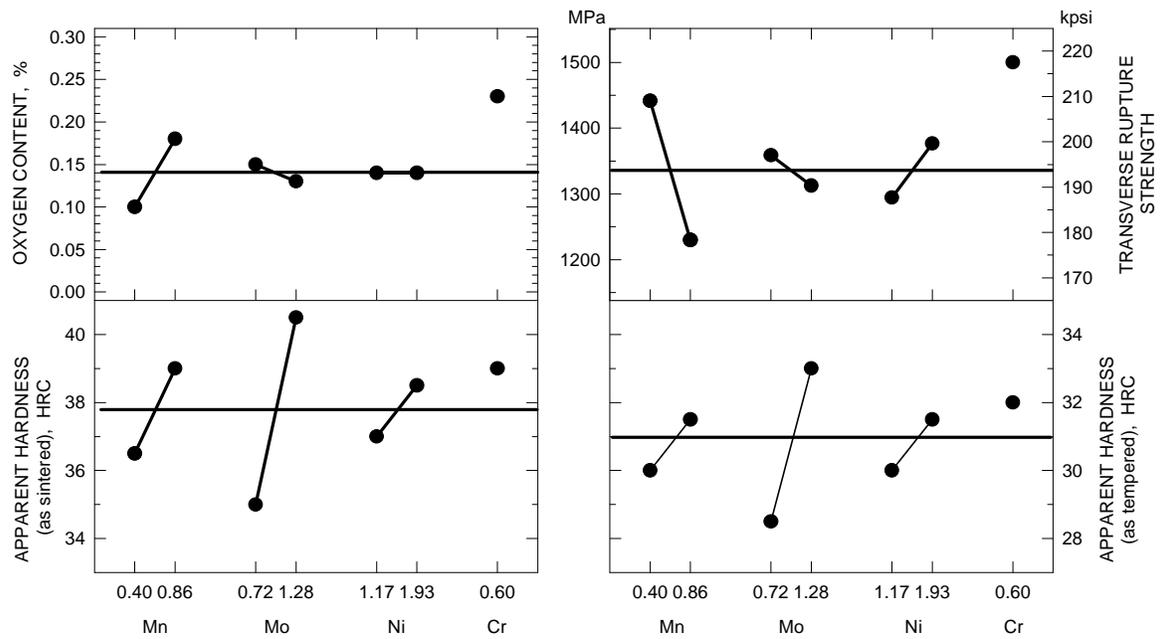
Figure 2. Mean effect of manganese, molybdenum, nickel and chromium on oxygen content of powder, transverse rupture strength, as-sintered apparent hardness and as-tempered apparent hardness.
