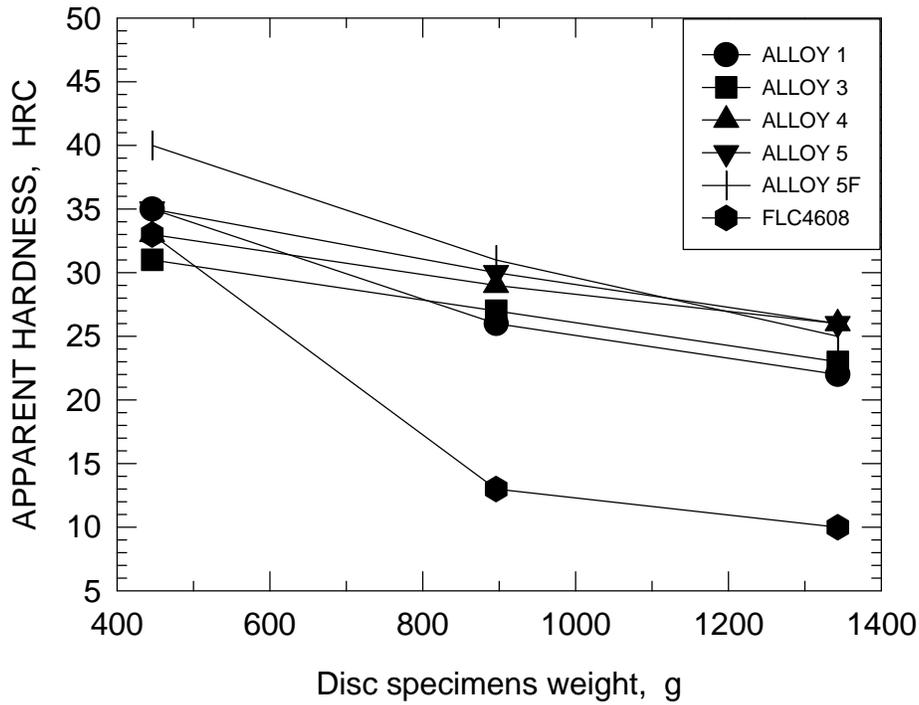
Figure 4. Effect of size on apparent hardness of the surface of disc specimens. (Average of 10 measurements on the top and bottom faces).
